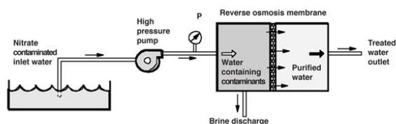
Figure 2. A schematic of the reverse osmosis process.
